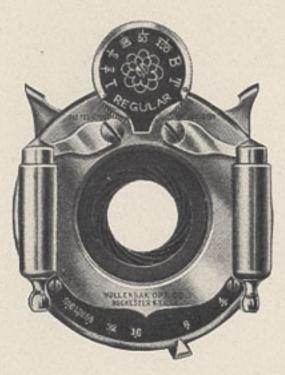
THE "Regular" is a double pump shutter of high grade, and in addition to the time and bulb exposures gives three different speeds of instantaneous and three automatic time exposures. At the top is a milled disc on which is an indicator, and to set the shutter for the desired exposure the disc is revolved until the indicator is opposite the proper figures on the dial. The shutter is set by pressing down the lever to the right and
