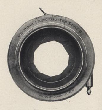
THIS shutter is made specially for use by professional photographers and is absolutely noiseless, as it has rubber cushions at all points of contact in the mechanism. The Studio Shutter has ten leaves, is constructed on the iris diaphragm principle and is made in two models. Style A being for use behind the lenses, is finished mat black, can be attached to board by screws and has focusing attachment. Style
