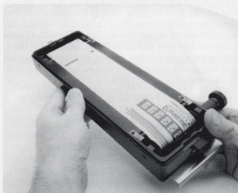
Fig. 6— Make certain film is aligned straight across the back of the film magazine without any kinks, and that it is centered on the take-up spool.
