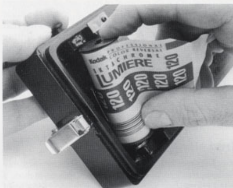
Fig. 5 — A roll of 120 film is installed in the compartment on the left. The film unwinds from the top and to the right.
