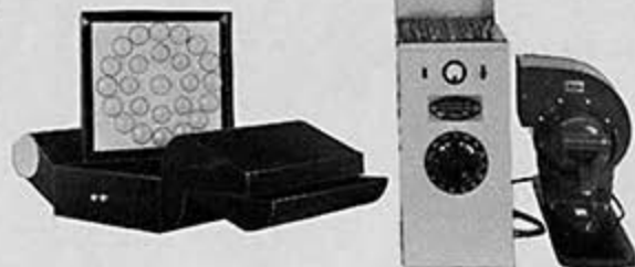
Diffused Incandescent Light Source with individual control for each bulb. Step-up transformer 3200° Kelvin (color temperature) with Variac and Voltmeter.
