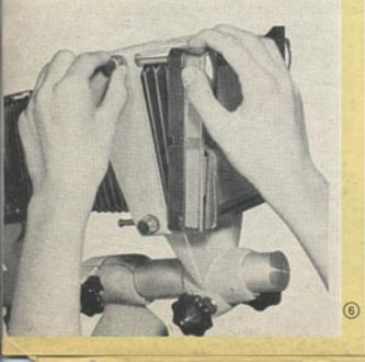
The Lens Standard is adjustable in four ways: (1) Height adjustment; (2) Lateral shift; (3) Lens tilt on the horizontal axis; (4) Lens swing on the vertical axis. The practical application of all camera movements is fully described in the LINHOF Technique Manual, and in LINHOF PRACTICE, available through your camera dealer. The extremely sturdy construction of the lens standard permits the use of heavy lenses (ill. 4)
