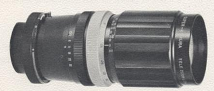
Diaphragm: Automatic and Click-Stops Minimum Aperture: f/22 Angle of View: 33° to 16° Closest Focus: 6' Filter Size: 58mm Length: 153mm Weight: 22-oz.
