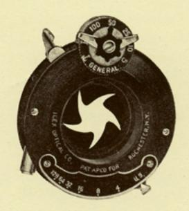
This shutter is a popular priced "general-use" shutter, strictly automatic in action and does not require setting. It may be operated either by finger-lever or wire release. The entire mechanism is controlled by one dial operating in either direction. It is similar to our Ilex Universal.
