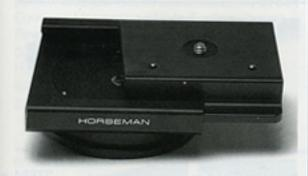
For quick, easy, yet secure mounting of camera on the tripod. Simply attach shoe to tripod, adapter to camera, then slide shoe into adapter until it locks in place. The shoe has spring-loaded stopper pins at both ends to secure the camera even when it is not yet properly locked in place. The two guide pins on the adapter determine the positioning of Horseman field cameras.
