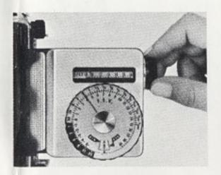
If the reading is too low and needle fails to indicate, move range switch to next higher sensitivity, eg. from 6-11 to 2-6 for low light level situations. Select the f/stop desired and make your exposure readings. If the light is too dim for the f/stop you desire to use, open up the lens or refer to the procedure described under 'methods for applied use'.
