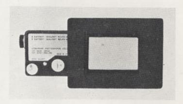
(7) Always turn meter OFF when not in use. The batteries are rapidly exhausted if the meter is left on for long periods of time.
