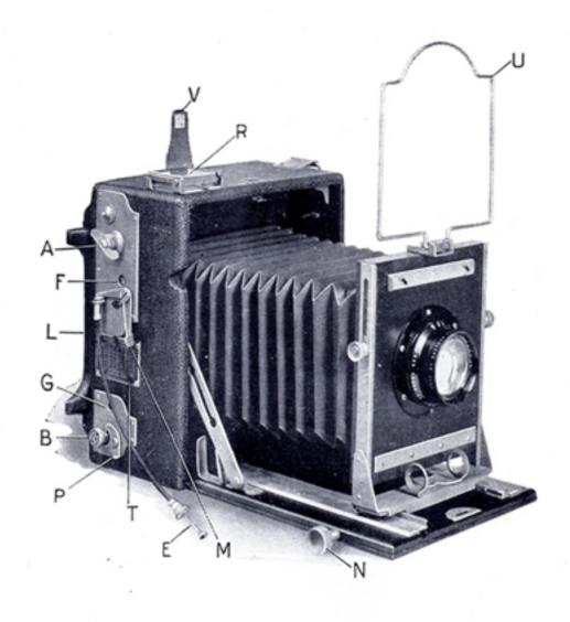
Open the camera by pressing the concealed spring at the top; swing the bed down until the spring-actuated side arms lock the bed in extended position. Grasp the front standard clamp and draw the lens standard out to the "infinity stop" fastened on the bed track.
