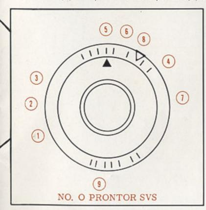
COUPLED EV SETTING: Lever (7). Press in and position to solid dot. This couples the shutter and diaphragm settings. In the coupled position, changing one scale setting changes the other. To uncouple and operate diaphragm and speed setting independently, return lever (7) to the open dot position by pressing in and down. CABLE RELEASE: Threaded Boss (2). Use tapered tip type cable release.
