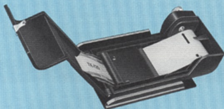
Daylight loading with either 120 or 220 rolls. Film counter automatically runs off paper leader after arrows on backing paper are aligned with windows in pressure plate.
