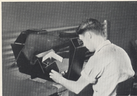
One of the steps in the manufacture of a B&L Photographic Lens is the examination of the glass used under polarized light. This reveals strain that escapes detection in ordinary light, but which would degrade the definition of the finished lens.
