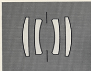
The B&L Process Apochromat employs four single lenses in combination. In this design a high order of correction is provided by relatively simple but extremely precise construction.
