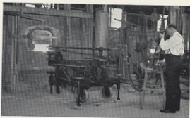
Every step in the manufacture of optical glass must be accurately and closely controlled. Temperature readings are made frequently to determine the completion of reactions and fusion.
